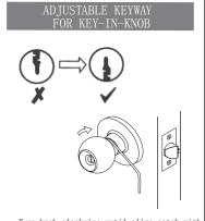
Turn knob clockwise until align catch with small hole. Insert key and turning counterclock about 45 degress. Use tool to depress catch and pull off outside knob. After turning 180 degrees, install again.
